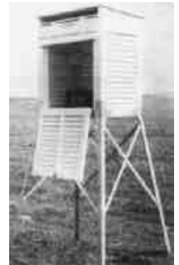
A Stevenson Screen is used to protect weather instruments from the elements.
