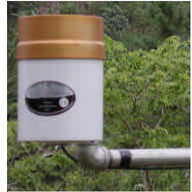
A rain gauge is used to measure rainfall amounts.
